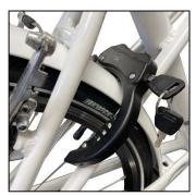
in the lock. If the rider wants to stop temporarily along their ride, they can engage the lock and remove the key. When the key is used to unlock the bike, the key is again trapped in the lock. When done using the bike, they simply lock the bike and return the key to the front desk. Since they can't get the key without the bike being locked up, this provides a level of assurance that the bike is secure when keys are returned.
